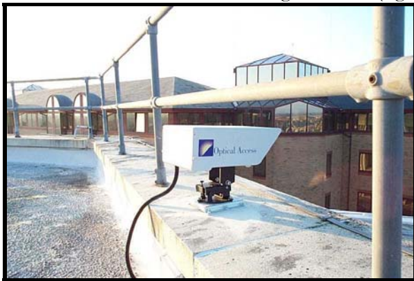
Figure 2.6: Parapet/Ledge Mounting (using JMP only)
